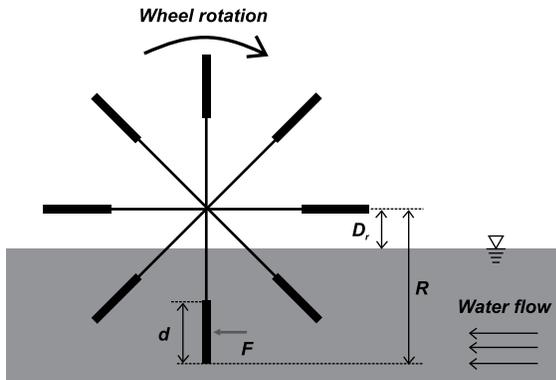
Figure 6. Side view of undershot waterwheel.
