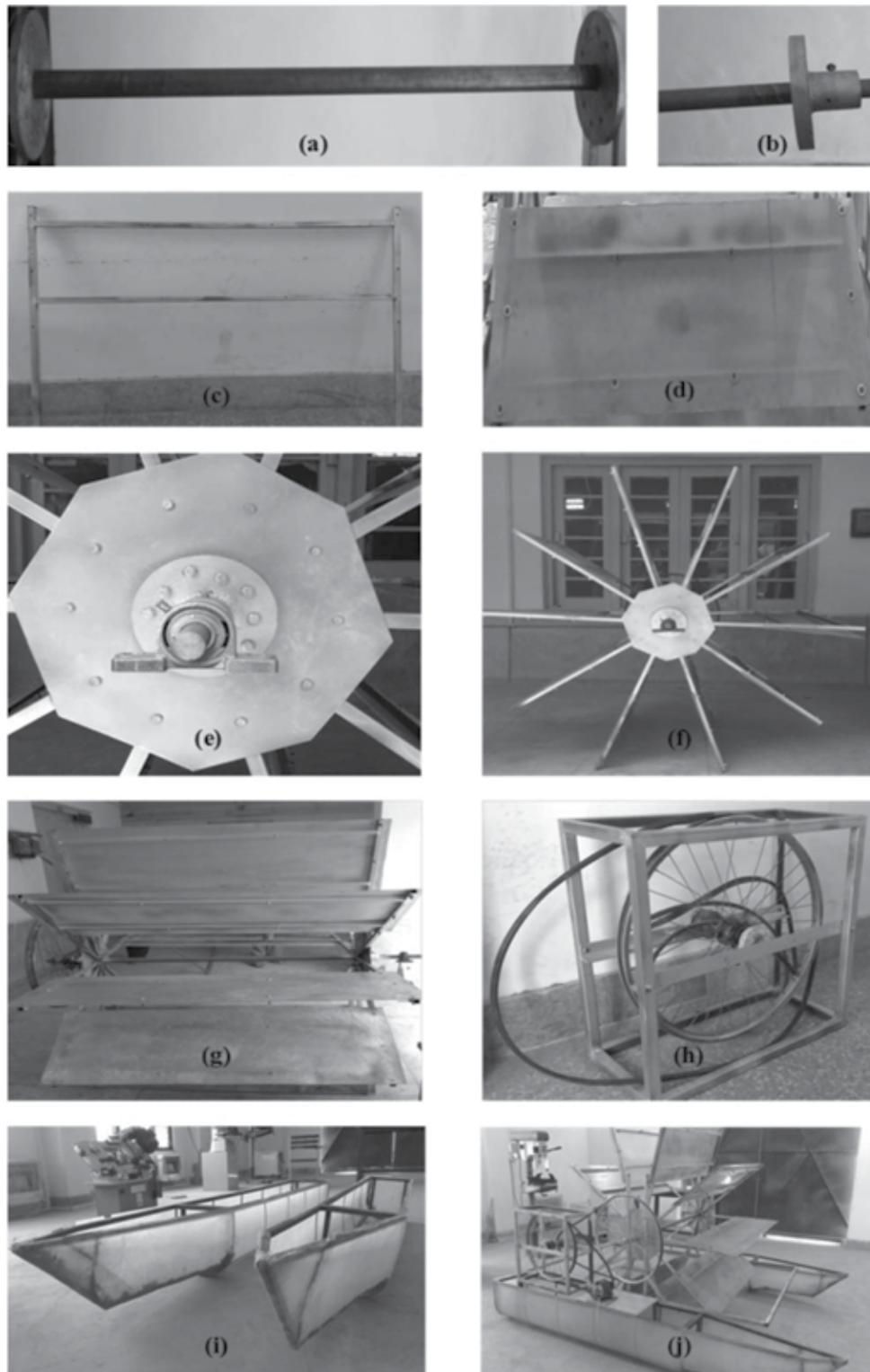
Figure 18. Fabrication of initial prototype floating waterwheel: (a) Shaft, (b) rotor collar, (c) blade frame, (d) blade made from fiber glass, (e) self-aligned roller bear on shaft, (f) fabricated rotor side view, (g) Fabricated rotor front view, (h) pulley box, (i) unfinished floats and (j) initial assembled prototype floating waterwheel.
