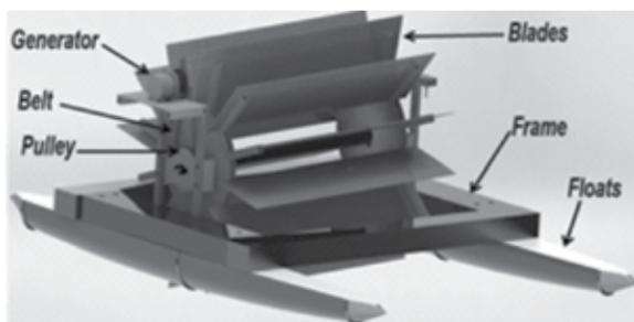
Figure 4. Solid model of floating undershot waterwheel.
