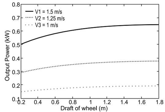
Figure 14. Variation in output power with draft of wheel
