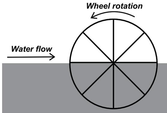
Figure 2. Schematic diagram of a Breast shot waterwheel
