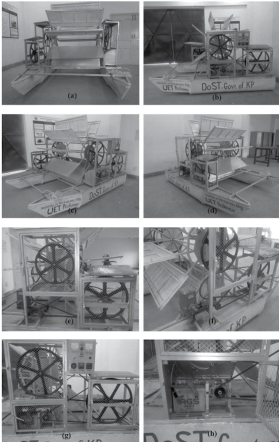
Figure 19. Fabrication of optimized prototype floating waterwheel: (a) Floating waterwheel front view, (b) side view, (c) right isomeric view, (d) left isomeric view, (e) pulleys and pump assembly, (f) pump close up, (g) pulleys and generator assembly and (h) battery and generator close up.
