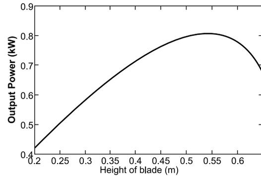
Figure 16. Variation in power with height of blade.
