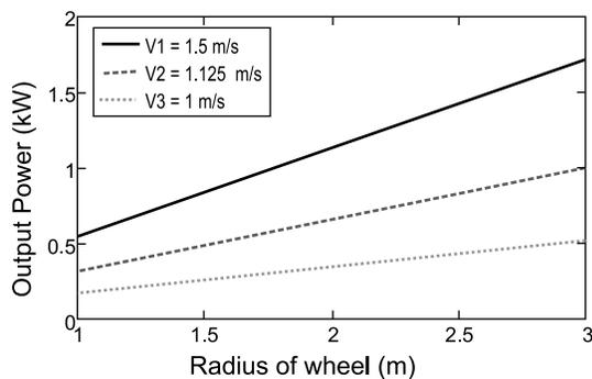
Figure 13. Variation of output power with radius of wheel.
