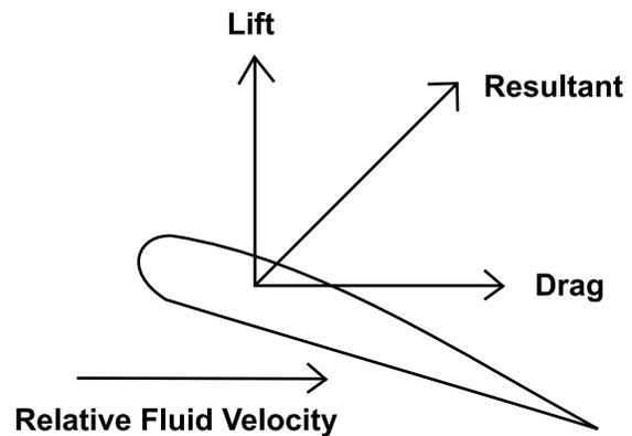
Figure 5. Flow over an airfoil.
