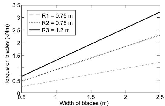
Figure 11. Torque as a function of blade's width at various radii of the waterwheel.
