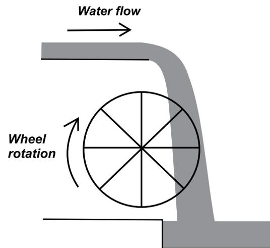
Figure 1. Schematic of overshot waterwheel.
